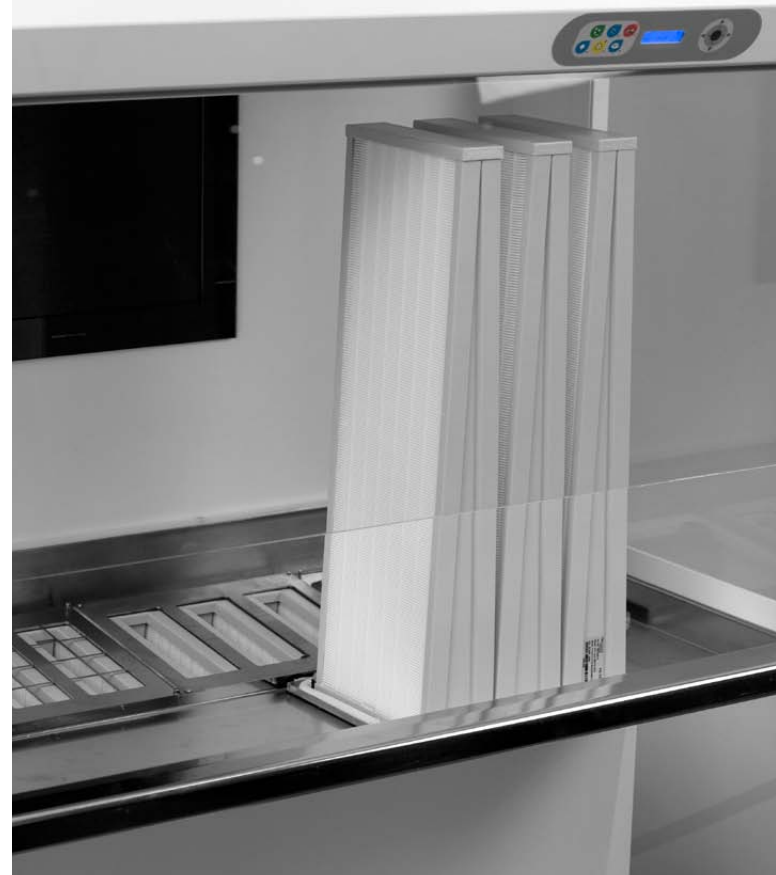
Triple Filter Cassette, already sealed, ready for removal via a Hazardous Waste bag.
