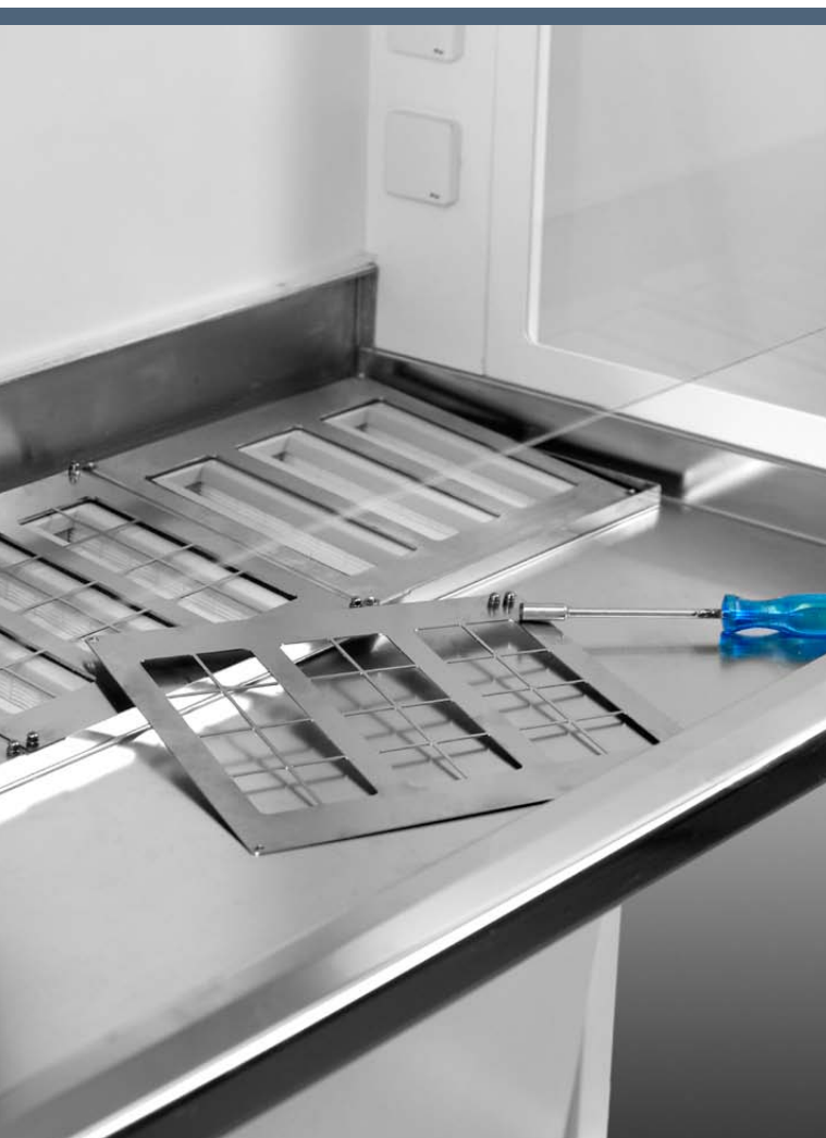
Removal of Filter Guard, prior to sealing the filters before removal.
